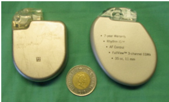
Figure: Two examples of ICD generators are shown with a two-dollar coin in between for size comparison.
